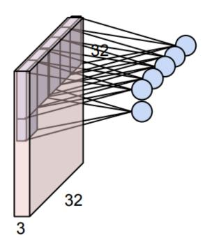
• An example of a 3-D convolutional layer with a  $5 \times 5 \times 3$  kernel (filter)
