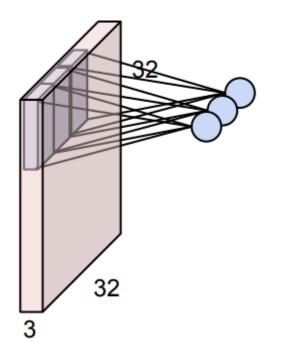
$\circ$  An example of a 3-D convolutional layer with a 5  $\times$  5  $\times$  3 kernel (filter)
