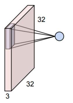
$\circ$  An example of a 3-D convolutional layer with a 5  $\times$  5  $\times$  3 kernel (filter)
