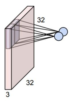
$\circ$  An example of a 3-D convolutional layer with a 5  $\times$  5  $\times$  3 kernel (filter)
